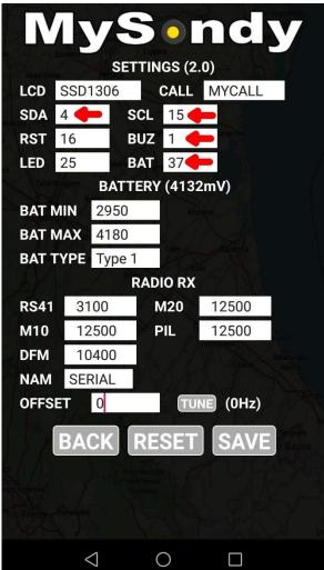
For a correct lecture of the battery voltage, it is necessary to add a resistive divider made of a 100k resistor, placed between Pin 37 and GND, and a 180K resistor, placed between Pin 37 and the positive wire of the battery.
